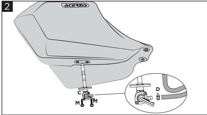
**Assemble the petcock (C) (including O-ring) using the appropriate screws (M). Fit the original clamp (D) on the pipe before connect it to the petcock.**
