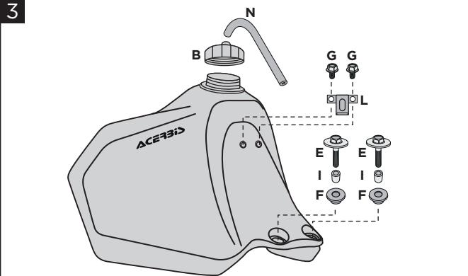
**Insert the tube (N) in the cap (B). Fix the bracket (L) using screws (G) and fix the tank on the frame using the rubbers (F), the bushings (I), and original screws (E).**
